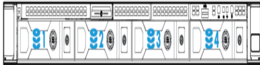
1-4 4 x LFF SATA/SAS/SSD Hot Pluggable Hard Drives Bays
